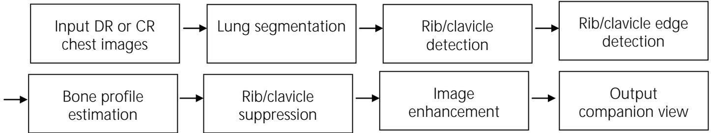
Figure 1: Image-processing chain to generate a bone-suppressed companion view
